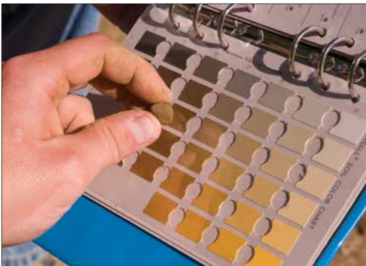
FIGURE 7—A Munsell chart is used to categorize the color of a soil.
